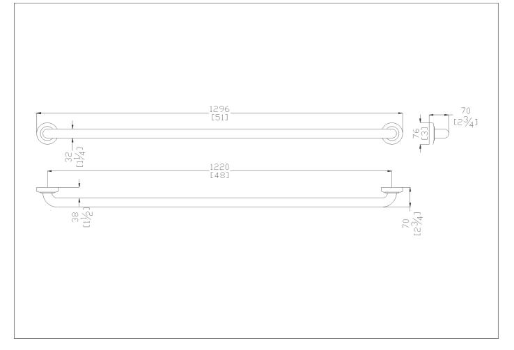
48" Center on center stainless steel grab bar with concealed flange plates. 1.25" diameter, 1.2mm wall thickness, 304 stainless steel.
