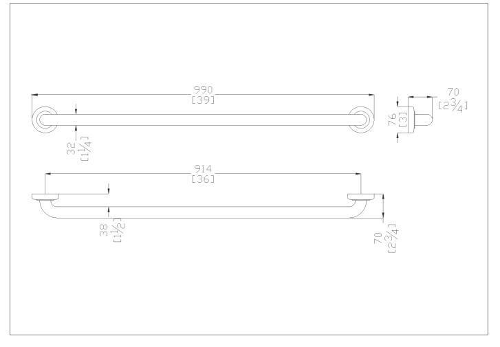
36" Center on center stainless steel grab bar with concealed flange plates. 1.25" diameter, 1.2mm wall thickness, 304 stainless steel.
