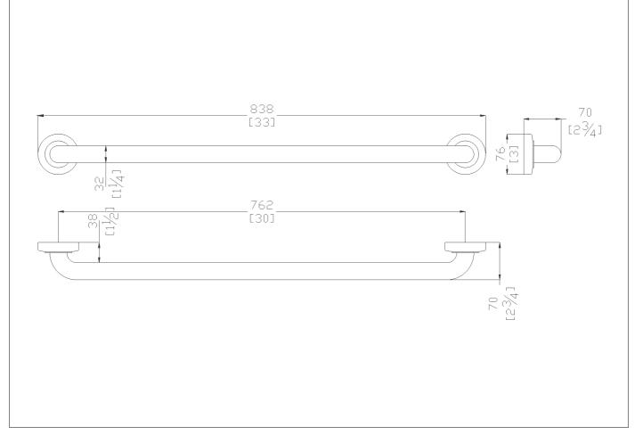
30" Center on center stainless steel grab bar with concealed flange plates. 1.25" diameter, 1.2mm wall thickness, 304 stainless steel.
