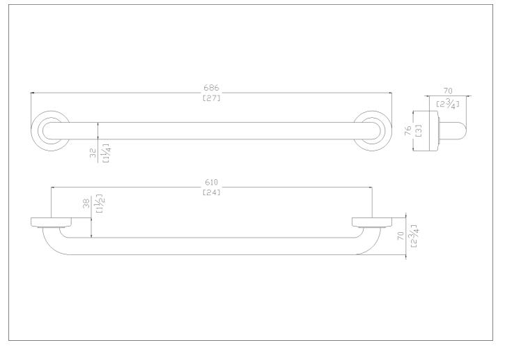
24" Center on center stainless steel grab bar with concealed flange plates. 1.25" diameter, 1.2mm wall thickness, 304 stainless steel.
