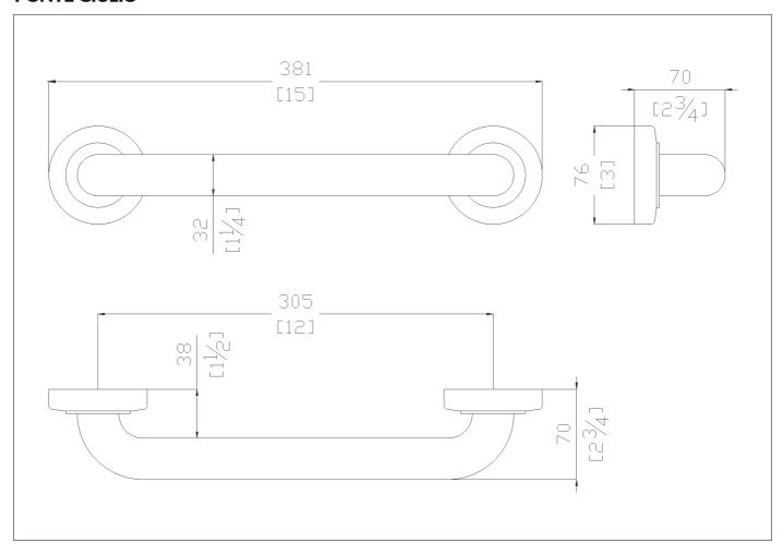
12" Center on center stainless steel grab bar with concealed flange plates. 1.25" diameter, 1.2mm wall thickness, 304 stainless steel.
