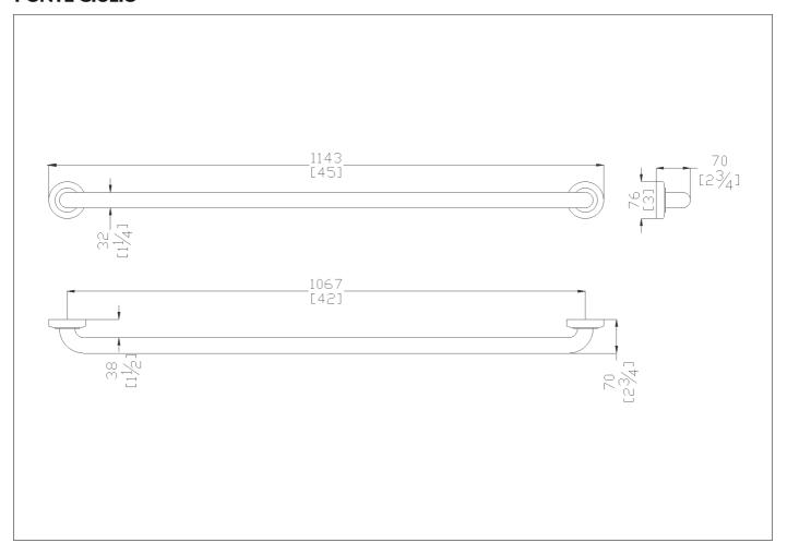
42" Center on center stainless steel grab bar with concealed flange plates. 1.25" diameter, 1.2mm wall thickness, 304 stainless steel.
