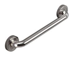
30" Center on center stainless steel grab bar with concealed flange plates. 1.25" diameter, 1.2mm wall thickness, 304 stainless steel.
