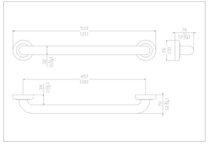
18" Center on center stainless steel grab bar with concealed flange plates. 1.25" diameter, 1.2mm wall thickness, 304 stainless steel.
