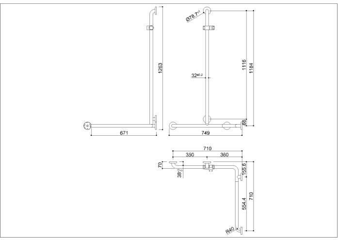
Safety handrail for corner installation with vertical arm, equipped with adjustable hand shower holder
