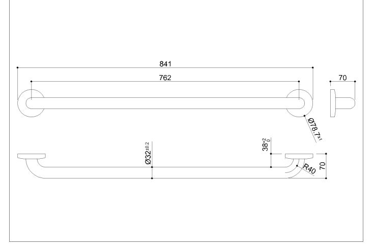
Straight grab bar made of seamless stainless steel AISI 304 pipe, with satin finish
