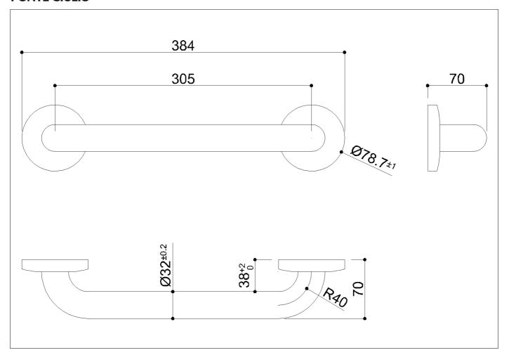
Straight grab bar made of seamless stainless steel AISI 304 pipe, with satin finish
