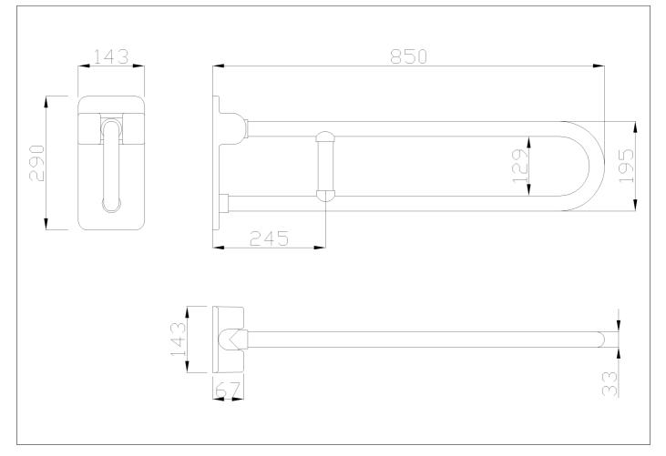
Folding grab bar with reinforced joint made of seamless zinc-plated steel pipe, coated with antimicrobial, biocompatible and warm-to-the-touch vinyl
