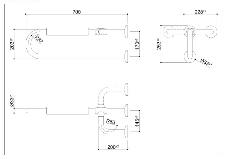
Fixed grab bar made of zinc-plated steel pipe, coated with antimicrobial, biocompatible and warm-to-the-touch vinyl. Equipped with soft armrest
