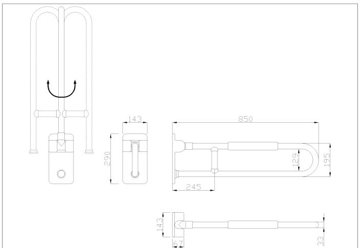
Folding and rotating grab bar with reinforced joint made of seamless zincplated steel pipe, coated with antimicrobial, biocompatible and warm-to-thetouch vinyl. Equipped with soft armrest
