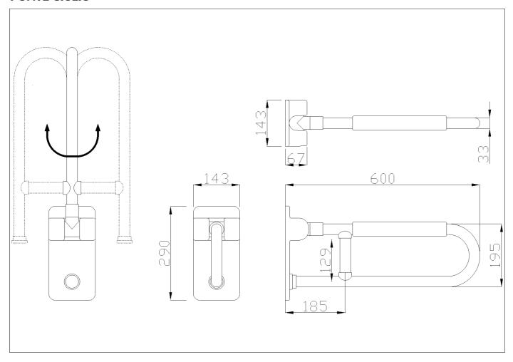
Folding and rotating grab bar with reinforced joint made of seamless zincplated steel pipe, coated with antimicrobial, biocompatible and warm-to-thetouch vinyl. Equipped with soft armrest
