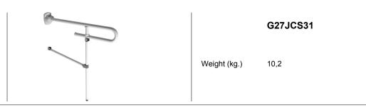
Safety folding grab rails with floor and wall support legs with stepless braking system, upper and lower position folding. Concealed wall fixing plate in stainless steel with polyamide cover. Base plate in polyamide for wall protection.
