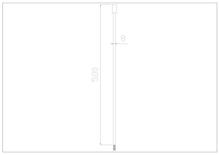
Ceiling support rod for shower rail made of  $\emptyset$  8 mm aluminium bar. Concealed wall fixing aluminium cylinder  $\emptyset$  15 mm. All the components are oxide satin external finish available only. The bar can be shortened when assembling it.
