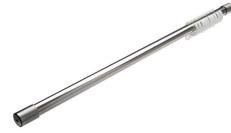
Flangeless straight shower curtain rail is manufactured of  $\emptyset$  32x1,5 mm stainless steel AISI 304 tube and comes complete with 16 curtain hooks. Installing the curtain rail is a cylinder system without seeing any screws, and adjusting the length of the rail can be achieved by using a pipe cutter or hacksaw.
