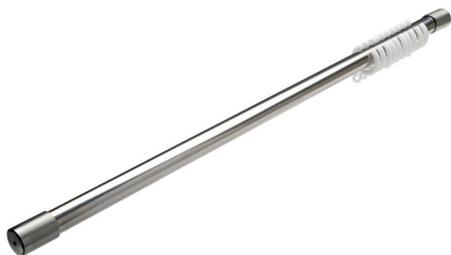
Flangeless straight shower curtain rail is manufactured of  $\varnothing 32 \times 1,5$  mm stainless steel AISI 304 tube and comes complete with 12 curtain hooks. Installing the curtain rail is a cylinder system without seeing any screws, and adjusting the length of the rail can be achieved by using a pipe cutter or hacksaw.
