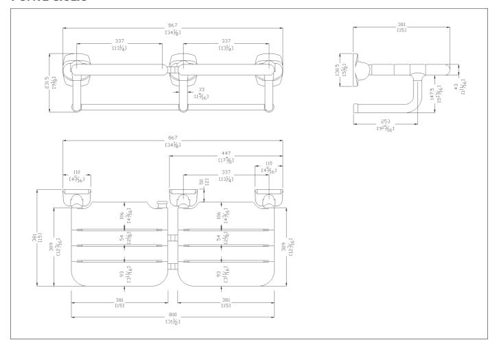
Double folding seat with nylon slats, made of stainless steel pipe, coated with antimicrobial, biocompatible, warm to the touch vinyl
