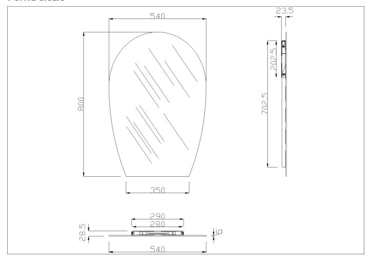
5 mm thick glass vertical mirror with bevelled edges.
