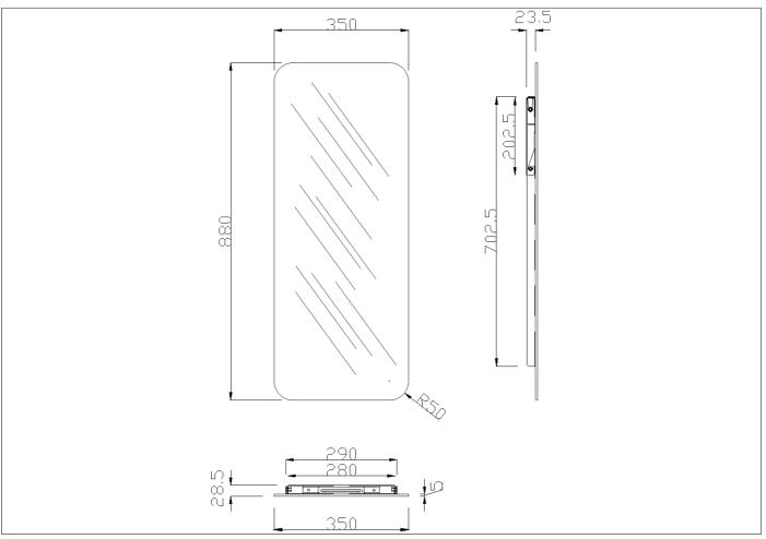
5 mm thick glass vertical mirror with rounded corners and bevelled edges.
