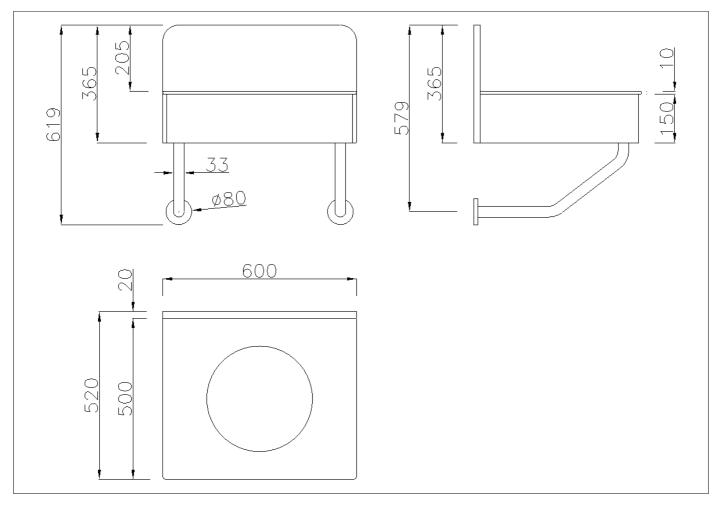
Wall hung wash basin supporting module, made of HPL panel, equipped with soft corner guards
