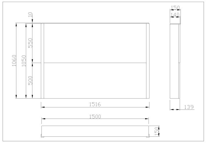
Equipped and inspectable module for the installation of 2 washbasins, made of HPL without decorations. Equipped with soft corner guards
