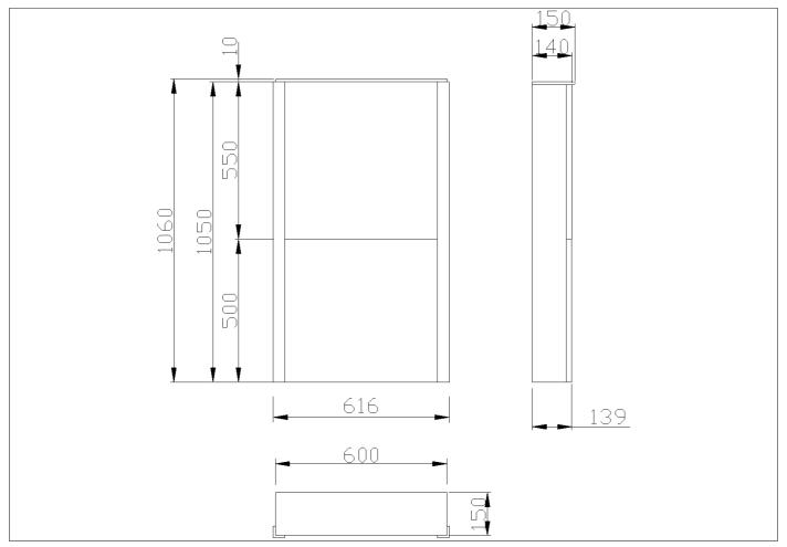
Wash basin supporting module, made of HPL panel, equipped with soft corner guards
